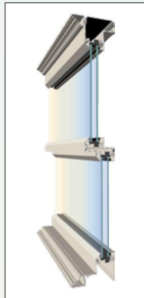
Cutaway view of sash, frame and glazing system found in the 1450 Series fixed windows installed on the Tuttle Courthouse Annex.
