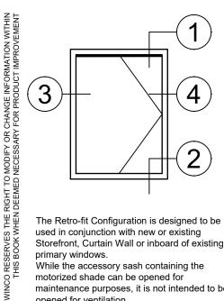
The Retro-fit Configuration is designed to be used in conjunction with new or existing Storefront, Curtain Wall or inboard of existing primary windows.
